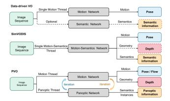
Figure 2. **Illustration.** Our PVO unifies visual odometry and video panoptic segmentation so that the two tasks can be mutually reinforced by iterative optimization. In contrast, methods such as SimVODIS [19] optimize motion and semantic information in a multi-task manner.
