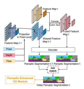
Figure 5. **VO-Enhanced VPS Module.** VO-Enhanced VPS Module enables feature tracking and fusion of different frames using the pose, depth, and optical flow information obtained from Visual Odometry. An online fusion module is included to better cope with occlusion challenges. The video panoptic segmentation results will be fed into the Panoptic-Enhanced VO Module.
