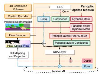
Figure 4. **Panoptic-Enhanced VO Module.** The Panoptic-Enhanced VO Module mainly feeds the 4D correlation volumes, the context information from the context encoder, and the flow information into the panoptic update module. The panoptic update module iterates N times to obtain better depth, pose, and optical flow estimation. The panoptic segmentation information is used to adjust the correlation weight and the optical flow is initialized as 0 and iteratively updated with the DBA layer.
