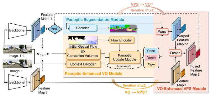
Figure 3. **Panoptic Visual Odometry Framework.** Our method consists of three modules, namely, an image panoptic segmentation module for system initialization (blue), a Panoptic-Enhanced VO Module (orange), and a VO-Enhanced VPS Module (red). The last two modules contribute to each other in a recurrent iterative manner.
