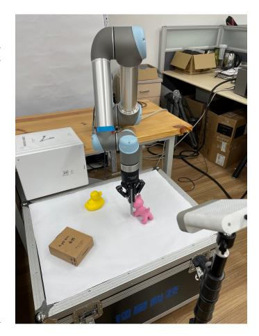
Fig. 1. A scene with several unseen objects. A fixed RGB-D camera is used to capture data, and a UR5 robot with a cylinder is used to poke the objects.
