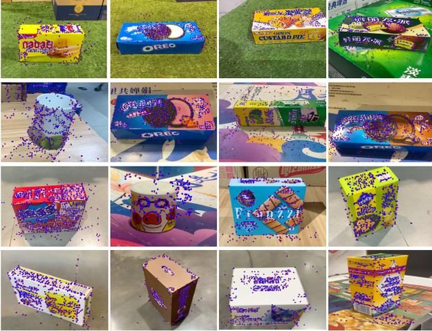
Figure 1. **Alignment quality across sequences.** Triangulated point clouds from one sequence are projected to images from another sequence of the same object. The quality of alignment can be measured by the differences between projected 3D points (in blue) and the original 2D keypoints (in red) on the images.
