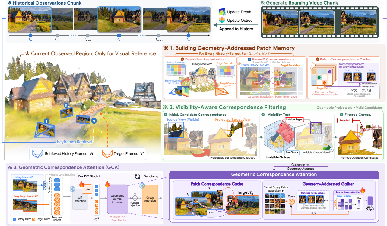
Figure 3. System overview. For each target chunk, GEAR constructs patch correspondences to retrieved history using per-frame geometry and filters occluded matches with the Invisible Octree. GCA then injects matched historical features into noisy target tokens during denoising, after which generated observations are appended to the history bank for continued rollout.
