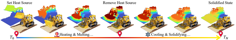
Fig. 13: Bidirectional phase-change editing. Controlled heating induces melting, while subsequent cooling drives solidification, demonstrating consistent thermomechanical evolution across phase transitions and enabling general thermophysical editing.
